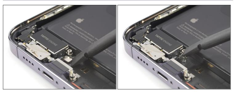
Use a spudger to disconnect the Taptic Engine by prying the connector straight up from its socket.
