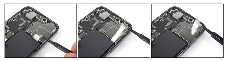
Using the same procedure as before, pull the third tab from underneath the battery. Try
