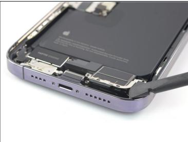
• Use the flat end of a spudger to pry up and loosen the loudspeaker from the bottom right corner of the phone.
