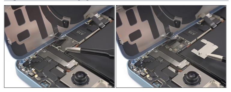
• Use a pair of tweezers to remove the charging coil connector cover.
