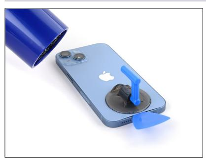
• Use a hair dryer to heat the left edge of the iPhone for 90 seconds or until the rear glass is slightly too hot to touch.
