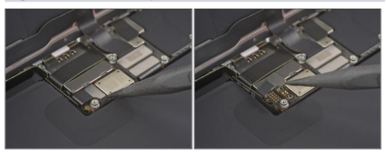
• Use the pointed end of a spudger to disconnect the battery cable by prying the connector straight up from its socket.
