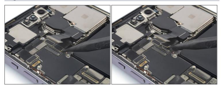
• Use a spudger to disconnect the wide lens cable by prying the connector straight up from its socket.
