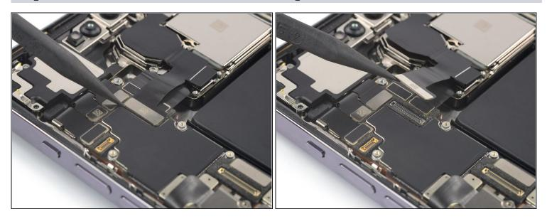
• Use a spudger to disconnect the ultra wide and telephoto lens cable by prying the connector straight up from its socket.
