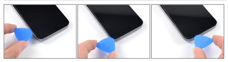
• Insert your pick underneath the top right edge of the phone. Slide it around the topright corner and half way across the top edge stopping right before the earpiece speaker cut-out.
