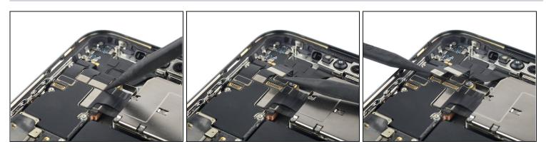
• Use a spudger to disconnect the camera and the sensor cables by prying the connectors straight up from their sockets.
