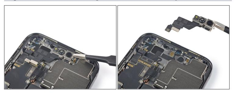
Use a pair of tweezers or your fingers to remove the front-facing camera and sensor assembly. If possible, turn on your device and test your repair before installing new adhesive and resealing.
