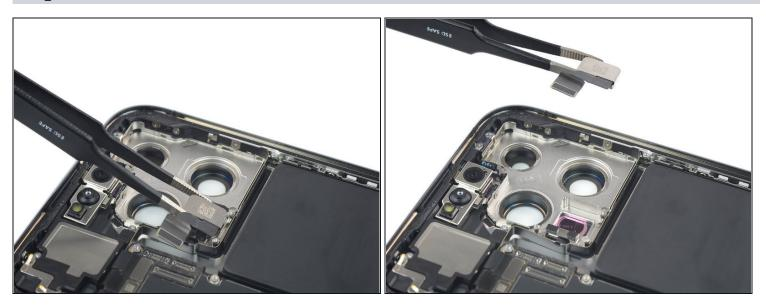
Use a pair of tweezers to remove the lidar sensor.
