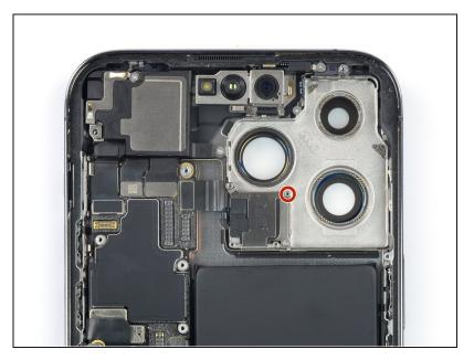
Use a standoff screwdriver to remove the 2.8 mm-long standoff screw securing the lidar sensor cover.
