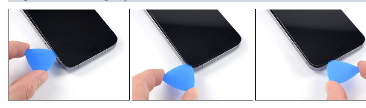
• Insert your pick underneath the top right edge of the phone. Slide it around the topright corner and half way across the top edge stopping right before the earpiece speaker cut-out.
