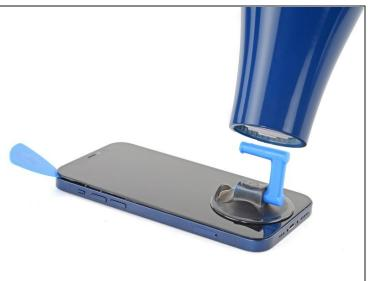
• Use a hair dryer to heat the left edge of the iPhone for 90 seconds or until the screen is slightly too hot to touch.
