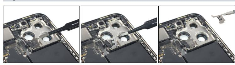
Use a pair of tweezers to remove the lidar sensor cover.
