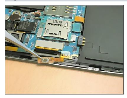
Detach the Power Key FPCB, that is stick to the bracket by a double-sided tape, using tweezers. Make sure to remove all remaining tape on the bracket.
