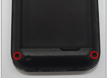
Unscrew 7 screws on the rear using a Phillips screw driver.
