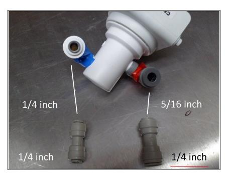
Here is a detail picture of the inlet and the outlet.
