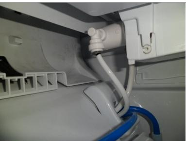
Behind the lowest drawer is an plastic panel, which can easy be pulled off. Now you can see the Water-reservoir for the Water Outlet. Also you can see on the right the hosing for the Waterfilter. There are no screws.
