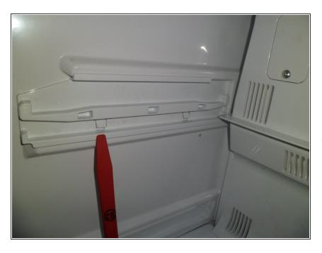
First take out three drawers. The Meat drawer is top, the Vitaminsafe is in the middle and the Freshzone is lowest. Between Meat & Vitaminsafe is a Bottom which is snaped in with clipse. Use a plastictool or a woodpiece to open the clips and remove the bottom. There are no screws.
