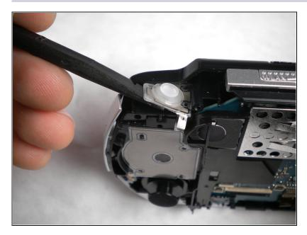
• Being careful not to break the ribbon cable, use the spudger to peel the adhesive button of the the 'L' trigger off the PSP.
