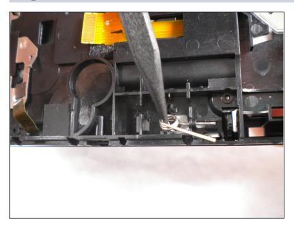
• Use a spudger and pull the spring out and remove it from the PSP.
