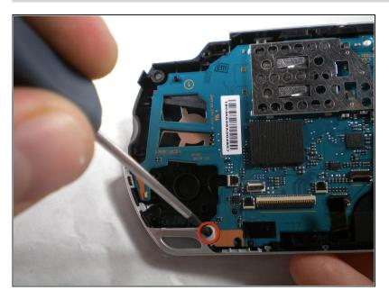
• Use a Phillips #00 screwdriver to remove the bottom left screw attached to the PSP
