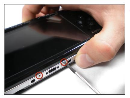
• Next, unscrew the two screws located at the top of the PSP.
