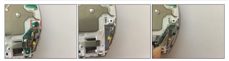
• Remove the screw located at the top of the power switch panel.
