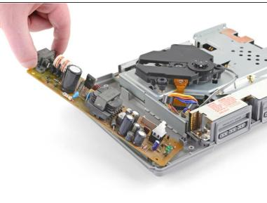
• Lift the outer edge of the power supply slightly, then rotate the whole power supply away from the small clip on its inner edge to remove the power supply.
