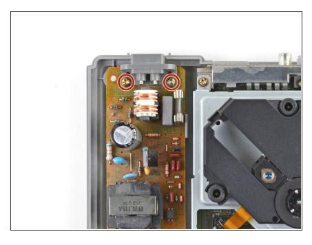
Remove the two 14 mm-long Phillips #1 screws securing the power supply to the bottom case.
