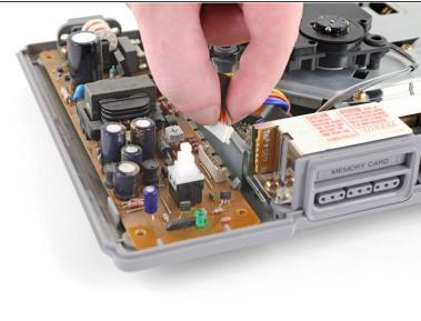
Pull the power supply cable straight up and out of its socket on the power supply to disconnect it.
