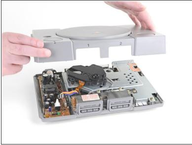
While holding the top and bottom halves of the console together, flip the console back over. Lift the top cover straight up to remove it.
