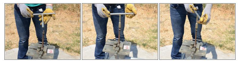
• Screw a T-handle onto the top of the pump rod. Tighten the T-handle up against the jam nut.
