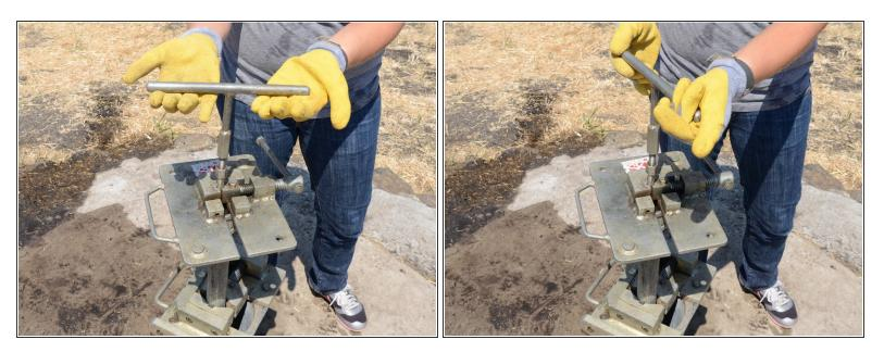
• Screw the T-handle onto the newly exposed top of the pump rod.
