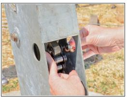
Remove the nut from the chain bolt.
