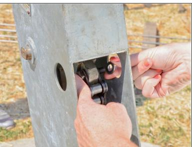
Remove the washer from the chain bolt.
