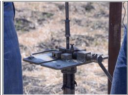
Attach and tighten the rod clamp a few inches below the first pump rod connection.
