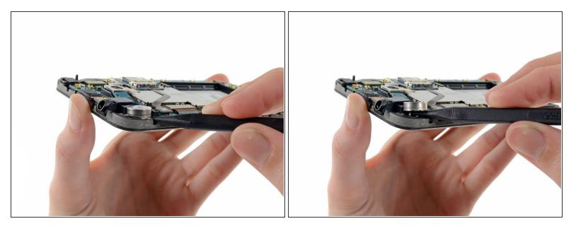
Insert the sharp end of a spudger into the gap in the corner of the midframe to free the vibrator from the adhesive.
