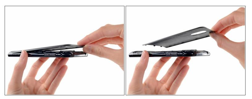
• Lift and remove the rear case.
