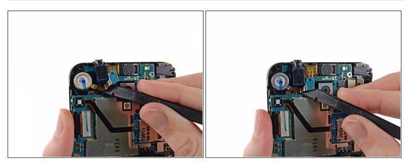
• Use the flat end of a spudger to release the headphone jack from the adhesive securing it to the midframe.
