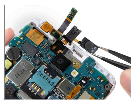
Use a pair of tweezers, or your fingers, to remove the headphone jack/earpiece speaker assembly from the display assembly.
