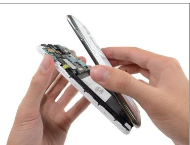
Remove the midframe from the display assembly.
