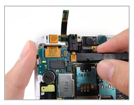
Use the flat end of a spudger to disconnect the headphone jack/earpiece speaker assembly connector.
