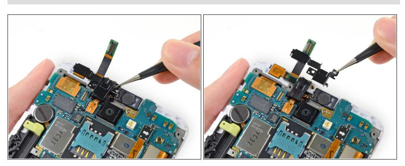
• Use a pair of tweezers, or your fingers, to remove the upper display assembly bracket.
