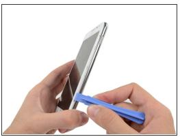
Slide the plastic opening tool down the seam.
