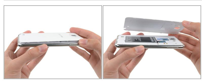
Lift and remove the rear case from the phone.
