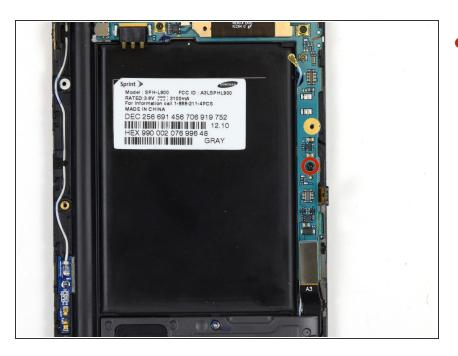
Remove the 3 mm Phillips #00 screw securing the motherboard to the display assembly.
