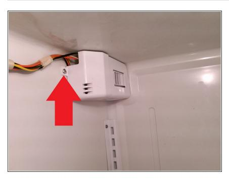
Unscrew the screw at the front of the diffuser cover. The diffuser itself will still be snugly in place.
