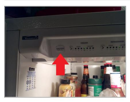
Turn off the fridge (on ours the switch is in the top left corner of the fridge.) Then unplug it or turn off the breaker.
