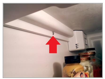
Remove the wire cover in the top left edge of the fridge. It's held in place by one Phillips head screw.
