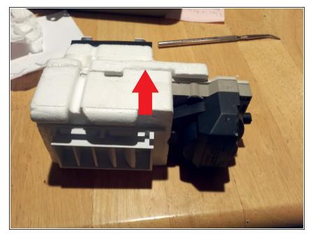
The diffuser assembly is a "nonserviceable" part. Unless you're stubborn like me. Gently cut open the foam along the glue line all the way around with a box cutter or sharp knife. Now remove the top half of the foam.
