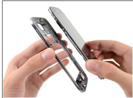
Remove the midframe from the display assembly.
