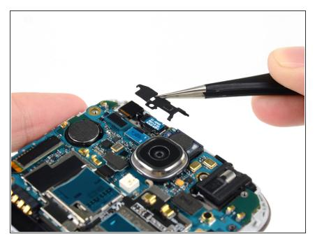
Remove the upper display assembly bracket.
