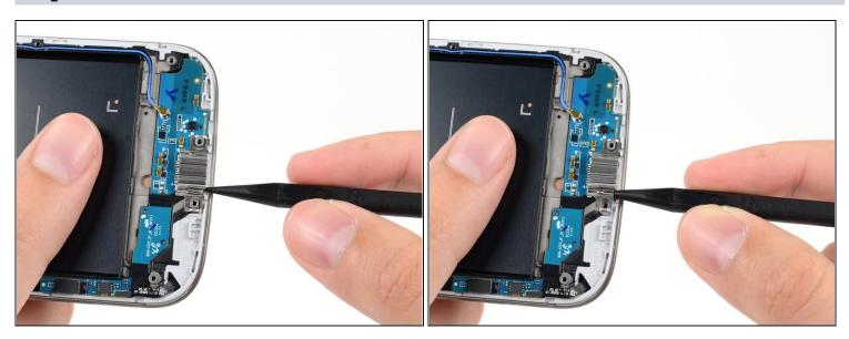
Gently insert the point of a spudger between the USB port and the USB port bracket to pry one side of the bracket off of its post.
