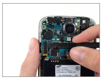
Use the flat end of a spudger to disconnect the USB board cable connector from the motherboard.
