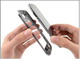
Remove the midframe from the display assembly.
