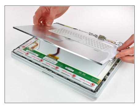
Carefully remove the thin steel LCD cover.
