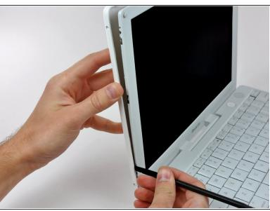
Working down from the upper left corner, use the flat end of a spudger to pry the rear bezel away from the left edge of the display.
