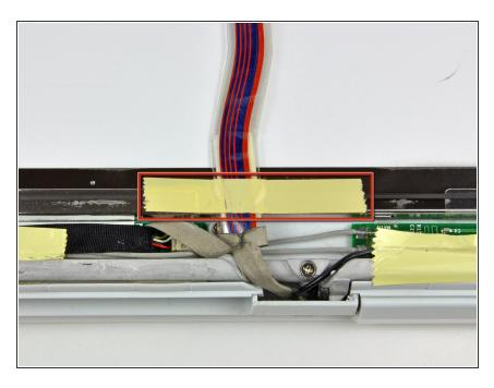
Remove the strip of yellow tape securing the display data cable to the metal LCD frame.
