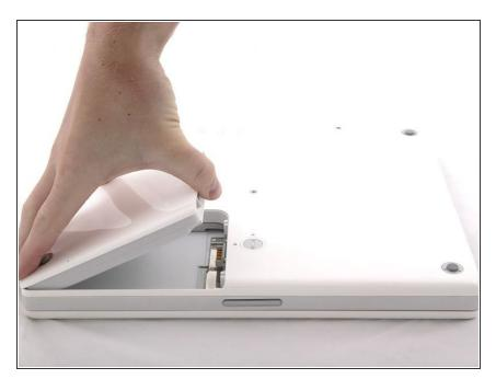
Lift the battery out of the computer.
