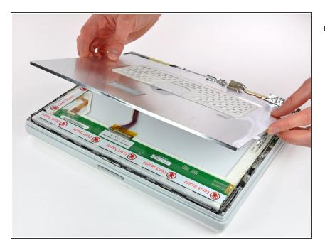
Carefully remove the thin steel LCD cover.
