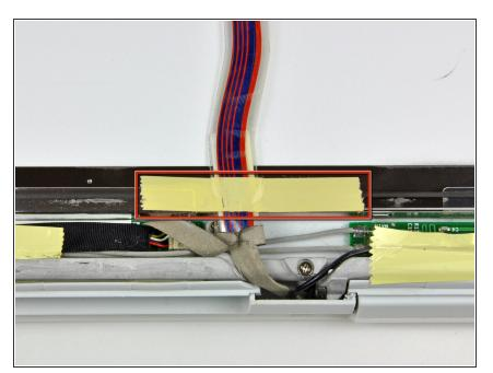
Remove the strip of yellow tape securing the display data cable to the metal LCD frame.
