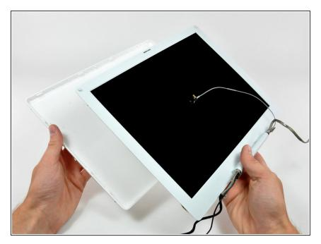
Lift the rear bezel off the display.
