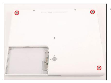
Remove the three newly-revealed Phillips screws.
