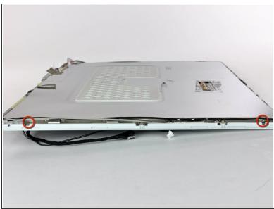
Remove the two Phillips screws securing each side of the LCD to the clutch hinge frame (four screws total).
