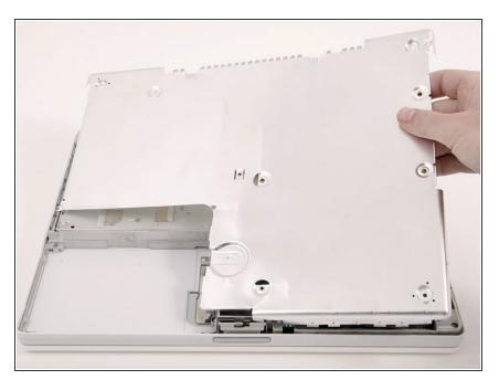
Lift the bottom shield off.
