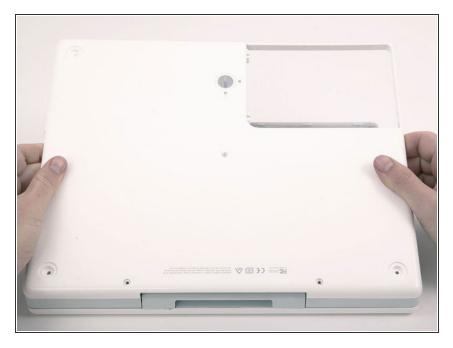
Once the front and sides of the lower case are free, turn the computer so that the back is facing you and pull the lower case up and toward you until the back tabs pop free (it may be helpful to jiggle the case up and down).
