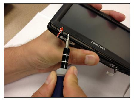
Insert the flat head screwdriver into the edge of the device. Using it as a lever, carefully pry the face-plate up.
