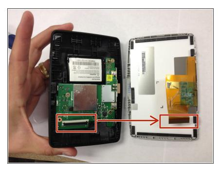
Carefully grab the ribbon cable with two fingers and pull the yellow ribbon cable upwards away from the motherboard.
