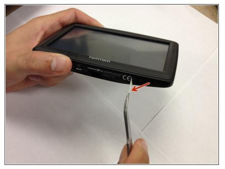
• Peel back the sticker, using the tweezers on the bottom of the device to reveal the two screws.
