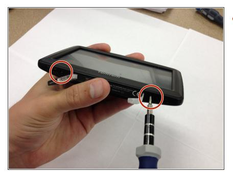
Re-insert the two T5 screws and tighten.
