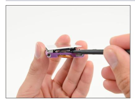
• Use a spudger to press the midframe screw tab up and out of the rear case.
