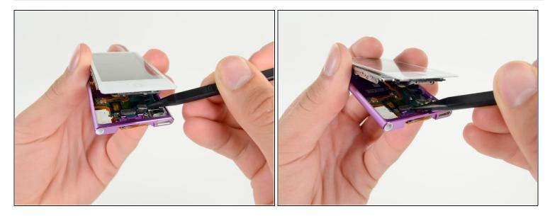
• Use a spudger to release the digitizer cable and display data cable connectors.
