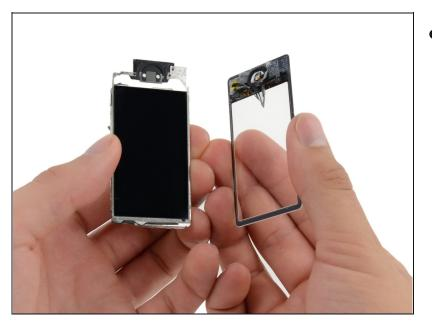
Once all of the adhesive has been released, gently separate the display assembly from the front glass/digitizer.
