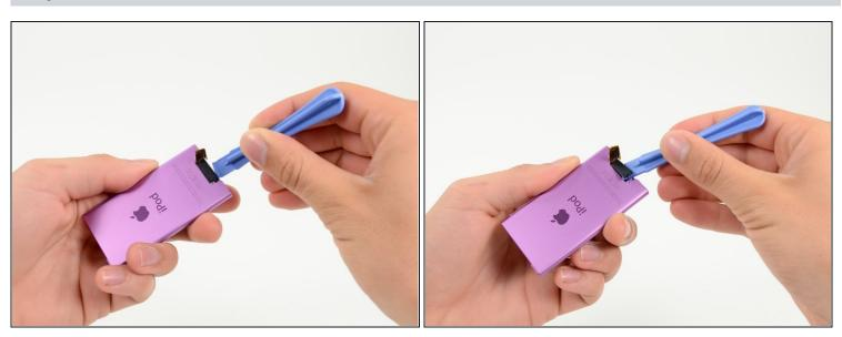
• Use a plastic opening tool to remove the black plastic spacer from the Nano.
