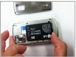
Find the slot at the bottom of the battery. Use a fingernail or opening tool to pry out the battery.
