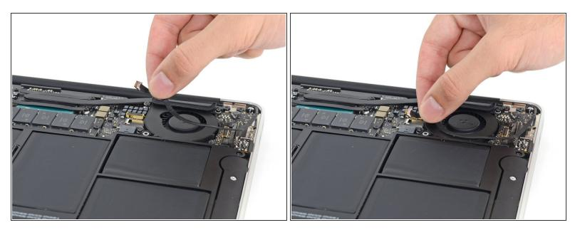
• Peel the iSight camera cable up off the adhesive securing it to the fan.
