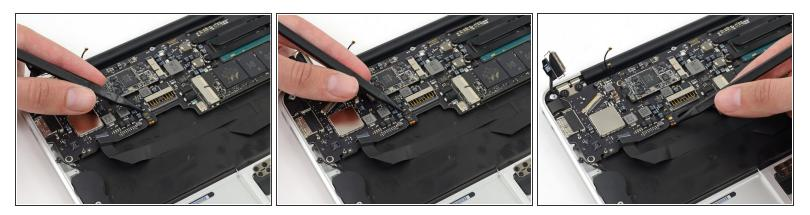
Use the tip of a spudger to flip up the retaining flap on the keyboard backlight ribbon cable ZIF socket.
