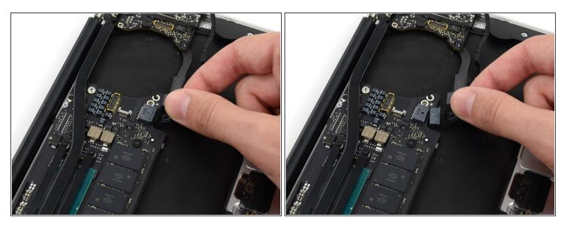
• Disconnect the I/O board by pulling the power cable away from its socket on the logic board.
