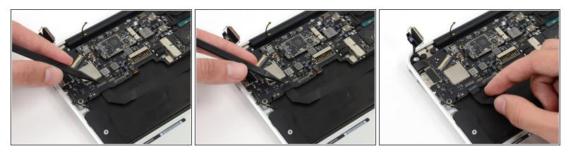
Use the tip of a spudger or your fingernail to flip up the retaining flap on the trackpad ribbon cable ZIF socket.
