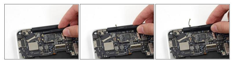
• Use the tip of a spudger to de-route the antenna cables from their notches in the logic board.
