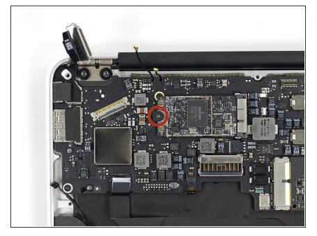
Remove the single 2.9 mm T5 Torx screw securing the AirPort/Bluetooth card to the logic board.
