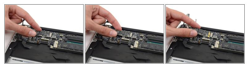
Slightly lift the free end of the AirPort/Bluetooth board and pull it out of its socket on the logic board.
