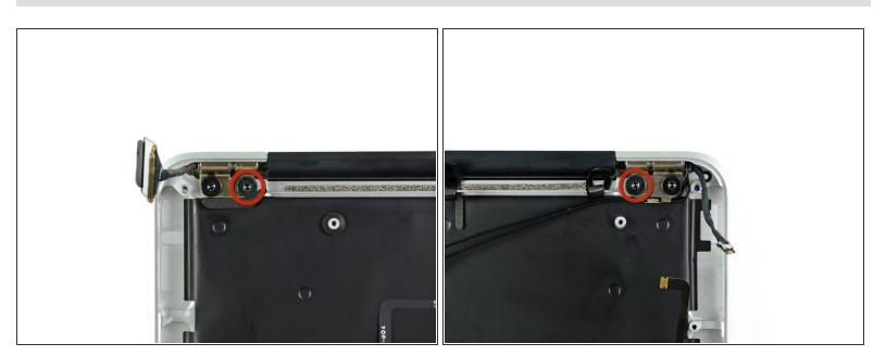
Remove the inner 4.9 mm T8 Torx screw securing each display hinge to the upper case (two screws total).
