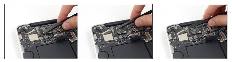
• Use the flat end of a spudger to pry both antenna connectors up from their sockets on the AirPort/Bluetooth card, and move them out of the way.
