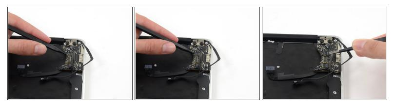
• Use the tip of a spudger to carefully flip up the retaining flap on the microphone cable ZIF socket.
