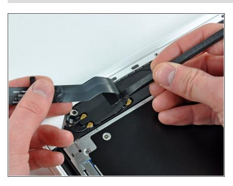
Use the flat end of a spudger to pry the AirPort/Bluetooth cable connector up off the right speaker.
