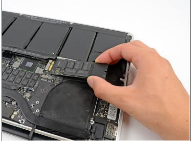
Slightly lift the rightmost side of the SSD and firmly slide it straight away out of its socket on the logic board.
