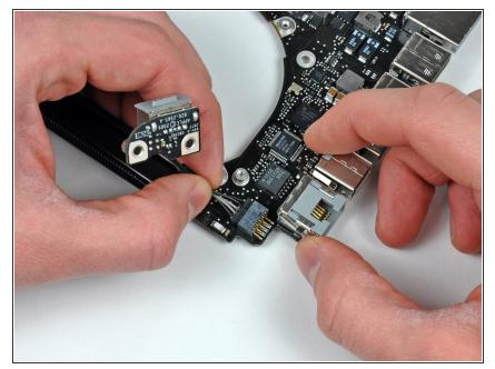
Disconnect the DC-In Board connector from the logic board by pulling it straight away from its socket.
