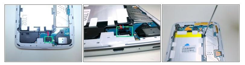
Once the back cover has been detached, you might want to detach the battery first to lighten the Tab's body when flipping around
