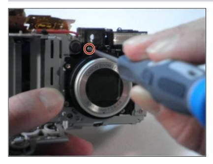
Remove the final screw directly under the left side of the viewfinder (on the lens side) with a Phillips #00 screwdriver.
