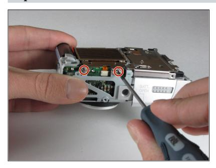
Remove the two screws from the bottom of the camera with a Phillips #00 screwdriver.
