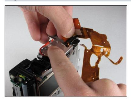
Gently pull the rest of the flex assembly away from the camera body until you reach the last connector.
