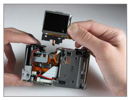
You have successfully removed the LCD screen. The camera is now ready for the replacement screen.
