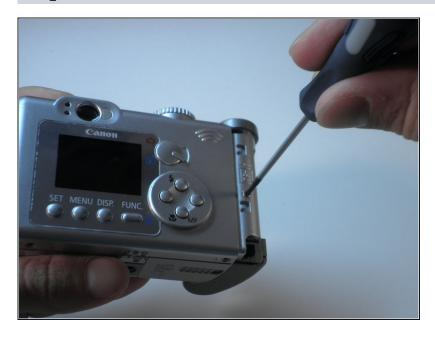
Remove the screw in the CF compartment with a Phillips #00 screwdriver.
