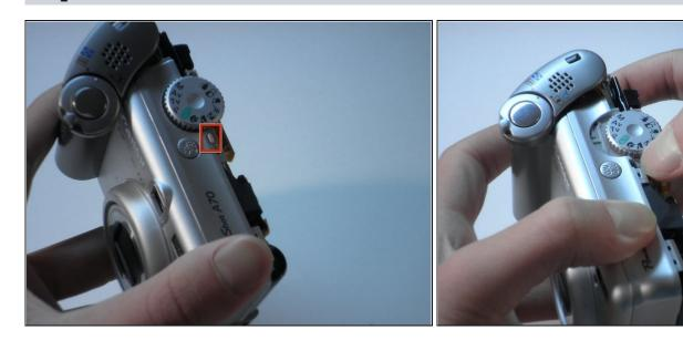
With your right thumb, pull back on the tab while using your left hand to pull the face of the camera away from the body.
