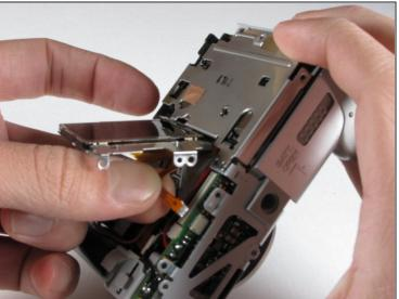
• Unplug the thin orange ribbon cable (located towards the bottom of the camera) by carefully pulling it away from the white connector.
