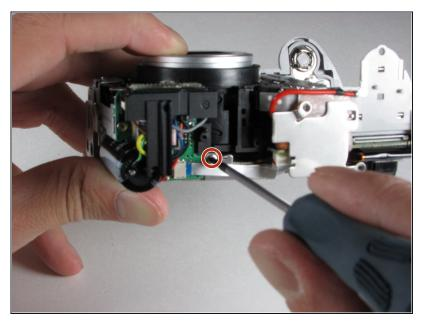
Remove the last screw located on the top of the camera with a Phillips #00 screwdriver.
