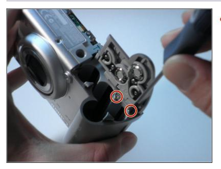
• Remove the two screws at the top of the battery compartment with a Phillips #00 screwdriver.
