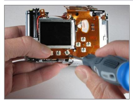
Using a Phillips #00 screwdriver, remove the one visible screw that attaches the flex assembly to the back of the camera.
