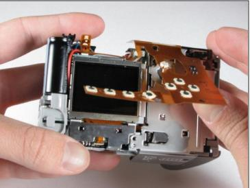
• Starting with the bottom-left corner (below the screen), lift the flex assembly away from the camera chassis.
