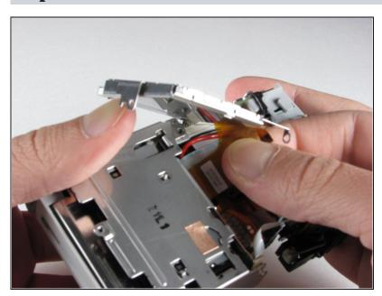
• Finally, repeat the previous step with the thick orange strip located on the side of the screen.
