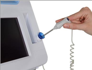
Grasp the temperature probe and pull it up to remove it from the monitor.
