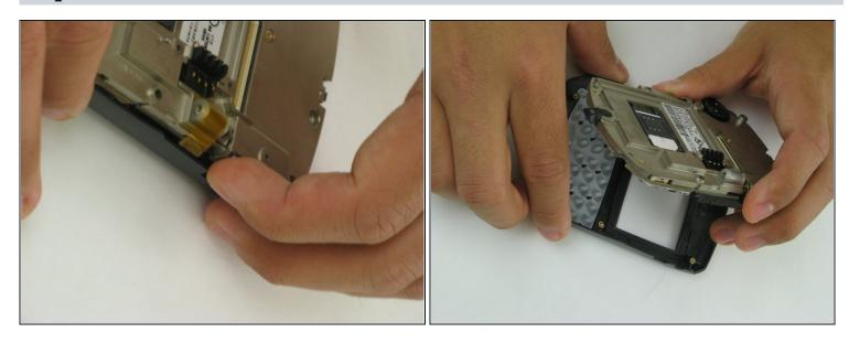
• Pull the metal plate away from the front panel of the cell phone.
