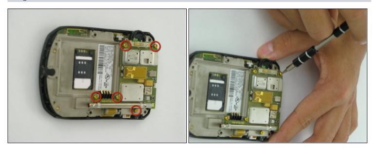
• Remove the indicated screws using a T6 Torx screwdriver.
