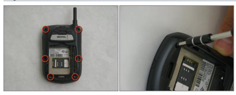
• Use a T6 Torx screwdriver to remove the 6 screws holding the rear of the phone.
