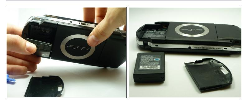
• Using your finger, remove the battery upwards from the system as shown.
