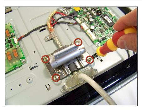
Remove these four screws holding down the base of the swing arm to the display and remove it
