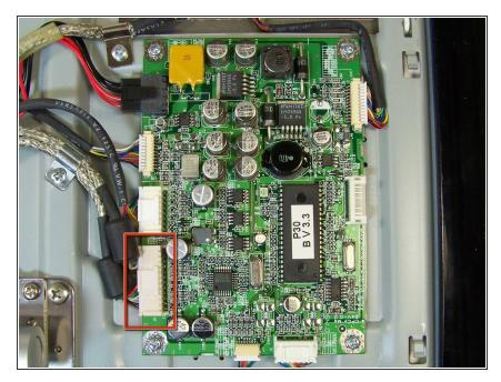
Remove the cable from the logic board that is connecting the USB port.
