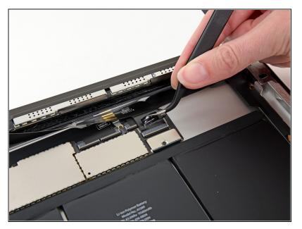
• Using the tip of a spudger, peel back the piece of tape covering the LCD ribbon cable connector.
