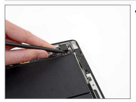
• Flip up the retaining flap securing the volume/power button ribbon cable connector to the headphone jack assembly board.
