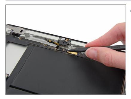
• Using the tip of the spudger, flip up the retaining flap on the microphone cable ZIF connector.
