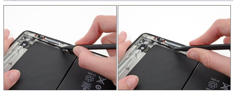
• Slide the tip of a spudger underneath the power & volume cables, releasing the adhesive.
