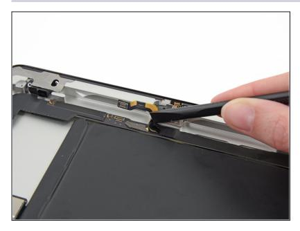
• Carefully move, but **do not remove** the front-facing camera ribbon cable aside with the flat edge of a spudger.
