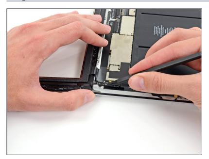
De-route the home button ribbon cable from its recess in the rear case.
