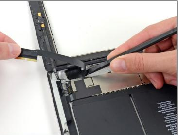
• Peel back the digitizer ribbon cable and use the flat end of a spudger to release the adhesive securing the cable to the rear aluminum case.
