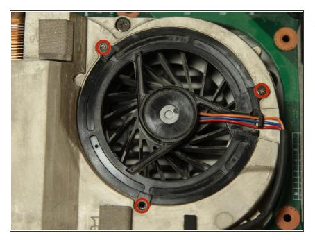
Remove the three 2 mm Phillips #00 screws that secure the fan to the motherboard.
