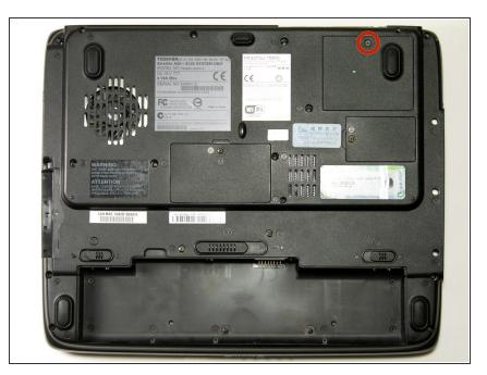
Remove the single 3mm Phillips #00 screw that secures the wireless card cover.
