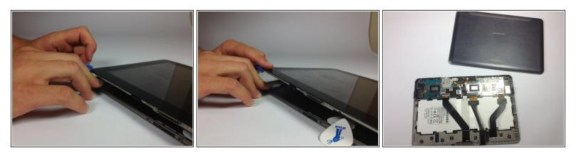
Using the plastic opening tools, continue to carefully run along the right and bottom edge, and then lift the screen from the back panel.
