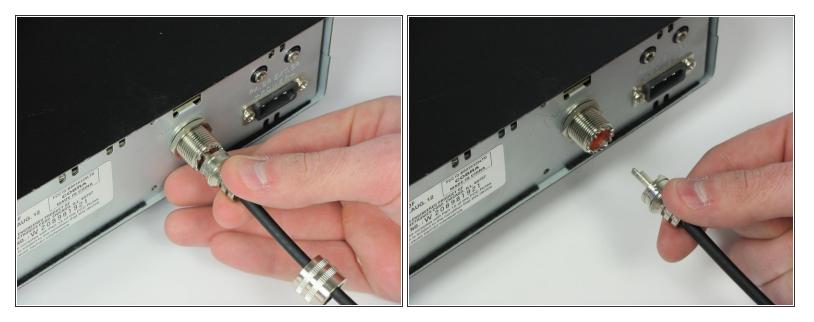
Gently pull the antenna cable to remove it from the back of the radio.
