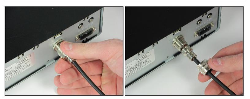
Unscrew the securing cap counterclockwise from the antenna connector.
