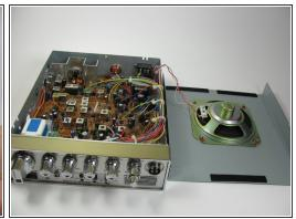
Match out for the wires connected to the speaker. These short wires will not allow you to move the cover very far.
