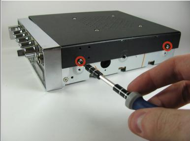
Unscrew the four 6.0mm Phillips head screws counterclockwise on the left and right side of the device that connect the remaining cover, using a #1 Phillips head screwdriver.
