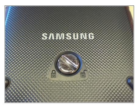
The first step, is remove the battery door. It comes with a security lock, that has to be on open position. Start opening from bottom, and releasing from the side edges.
