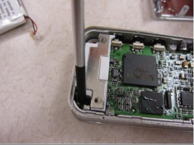
Using the philips screwdriver, remove the two screws on the mother board.
