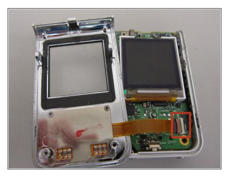
After opening the front cover you will see and electric ribbon connecting the buttons to the mother board.
