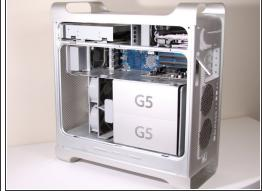
• Remove the air deflector (the clear plastic cover) by pulling on the handle.
