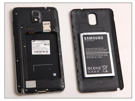
Turn the device off and use your finger to remove the back cover and battery. The Galaxy Note 3 battery is removable, making it easy to remove it without any tool.
