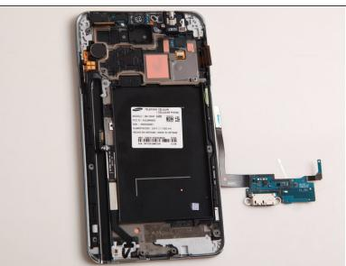
Use spudger to remove the USB board with proper strength because the USB board is stuck with glue.
