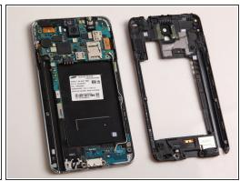
Pull out the S pen and use spudger to release the back chassis. Then the chassis is separated from the rest of the device.
