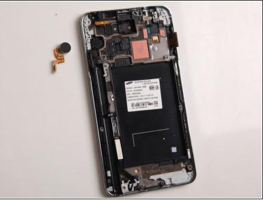
Use screwdriver to pry out the vibrating motor. Please be noted the motor is adhered to the front chassis and connected with the power button. Please lift it up carefully to avoid damaging the power button cable.
