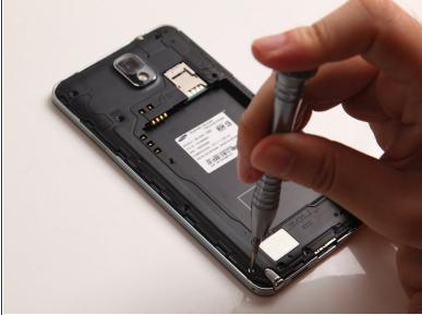
The back chassis is fastened by twelve Philips screws, so we have to undo the screws with the Philips screwdrivers.
