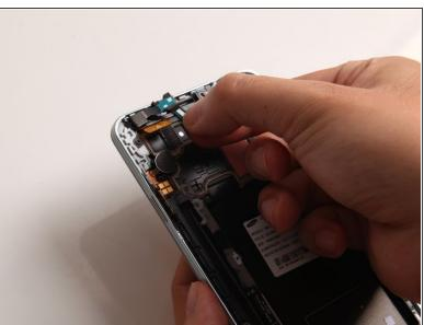
Remove the small metal bracket covering the front facing camera and sensor cable. Then remove the front camera and sensor cable.
