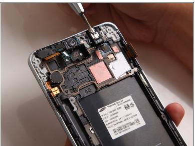
Undo the screw used to fasten the earphone jack and earphone and remove them.
