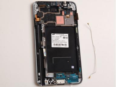
Use plastic case to release the antenna cable clips and remove the antenna cable.
