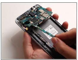
• Disconnect seven cable connectors to remove the mainboard. Then the board is free.
