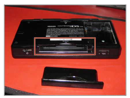
On the front edge of the Nintendo DS between the headphone jack plug and volume controls remove the plastic insert (or cartridge) from the lower slot (Slot 2).
