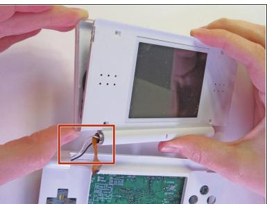
Unscrew the four Phillips-head screws and remove the top panel.
