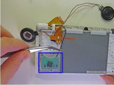
• Carefully remove the two speakers and the green wireless card from the top panel.
