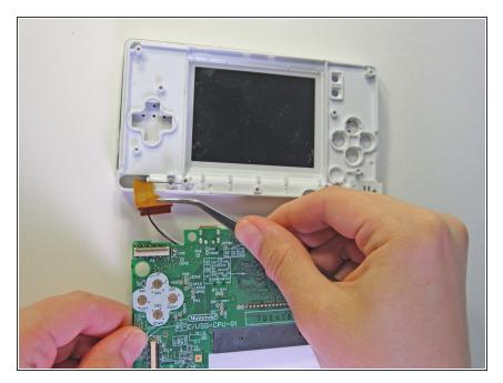
Using one finger nail or the plastic opening tool, carefully lift the brown securing flap of the connector. Then disconnect the ribbon cable that connects the logic board to the upper screen.
