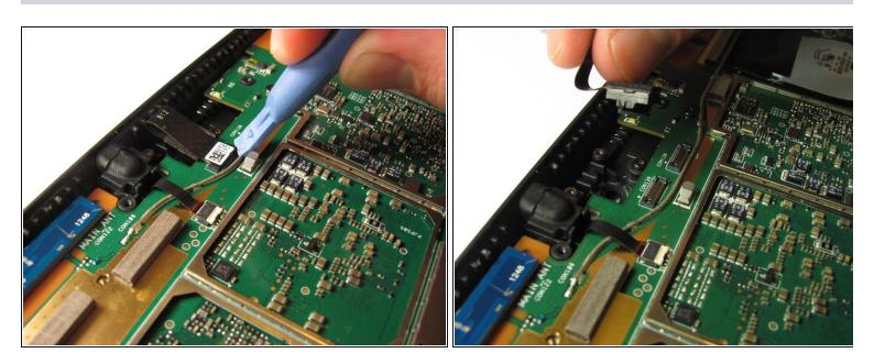
• Use the plastic opening tool to pry out the back camera.
