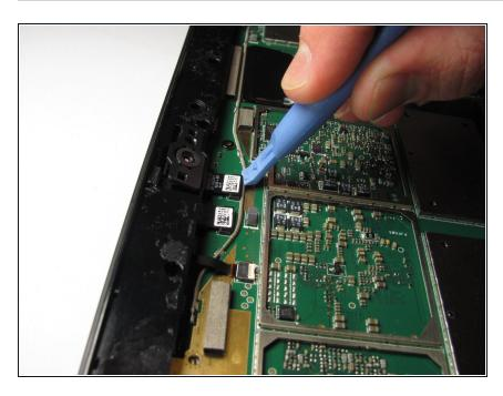
Use the plastic opening tool or fingers to pry out the front camera.
