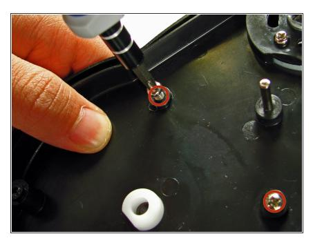
Using Phillips #2 screwdriver, unscrew two 12.7-mm screws in the middle of the base.
