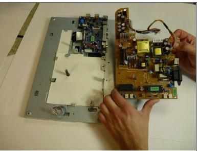
Lift the brown power supply board off of the frame and set it aside.
