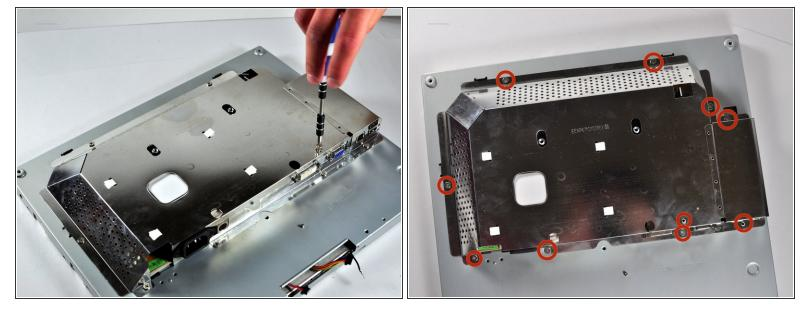
Unscrew the 10 5mm Philips PH2 screws holding the metal casing to the monitor.
