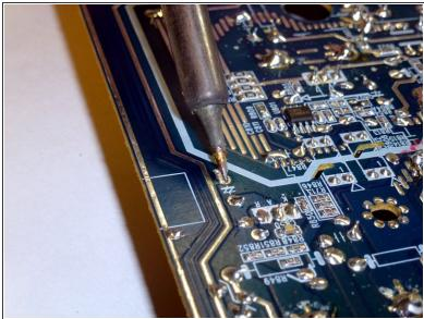
Use a <u>Soldering Station</u> and Desoldering Braid to remove the solder from the two joints.
