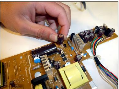
Remove the capacitor from the board, you may need to straighten out the leads before you can take it out easily.
